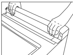
6. Remove the kick plate by pulling it outwards and upwards.
