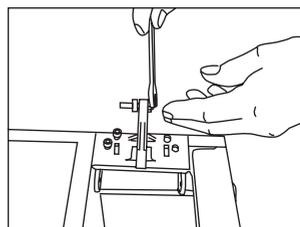
7. Remove the screws holding the lower hinge in place. Turn the pin on which the door was mounted so that it points in the opposite direction. Rotate the hinge through 180° and refit it on the opposite side of the appliance.
