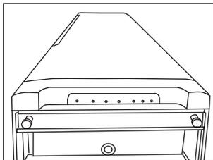
1. Lay the appliance on its back with the door uppermost.
